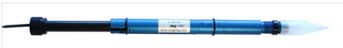
Figure 3: Microsensor mounted in the Microrespiration guide.
