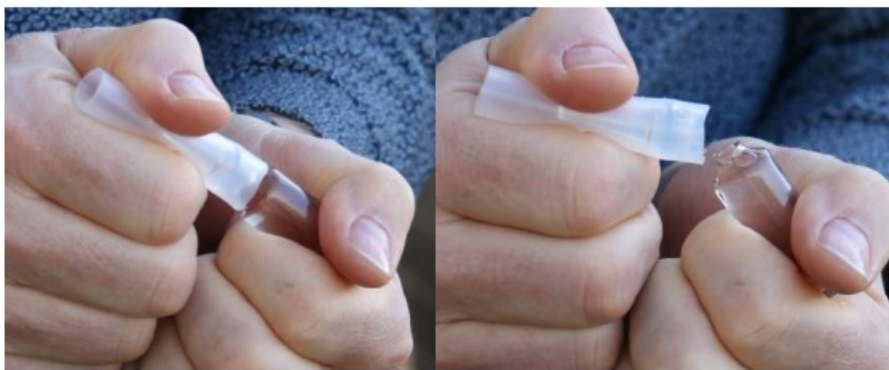
Figure 2: Open the ampoule. Leave the tubing on for protection.
