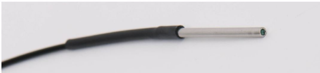
Figure 7: Optical oxygen sensor, Optode, in the Opto-3000 design.
