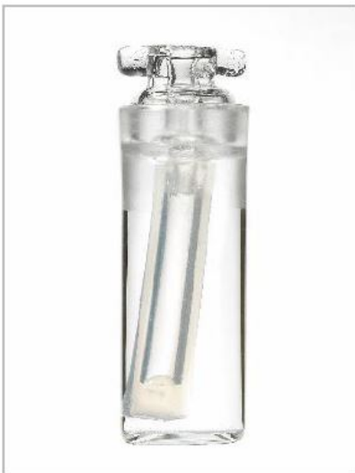
Figure 5: Zero calibration chamber (MR-Ch O-calibration). The zero solution is outside the silicone tubing and pure water is inside. The oxygen in the water inside the tubing diffuses through the silicone tubing into the zero solution where it is consumed.
