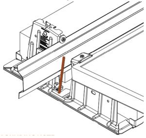
Ilsco SGB-4 Solar Grounding & Bonding
