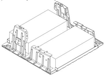
**WIND DEFLECTOR:** 18G G180 steel wind defl ector aids in ballast reduction and provides fi re mitigation. A 1/4" – 20 stainless steel bolt and fender washer (1.5" O.D) are associated hardware for wind defl ectors. **NOTE:** U-Nuts come in packages separate from defl ector hardware.
