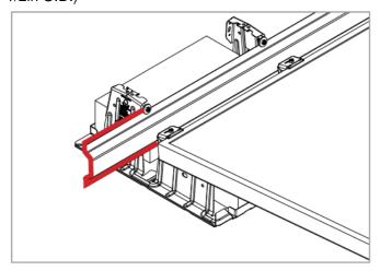
TYPE 1, 29, & 30: Install wind deflectors on North edge of array.
