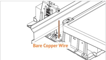
**BONDING JUMPER NOT REQUIRED**, due to integrated bonding/grounding path throughout module frames/bays around this location.
