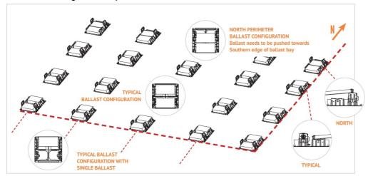
**SOUTHERN EDGE MODULE PLACEMENT:** Each bay has two spacing options, select the appropriate tab according to layout requirements.
