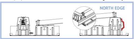
TYPE 2: Install wind deflectors on all perimeter modules within array
