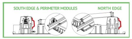
NOTE: Wind deflector should be secured to supplemental bay by two hardware kits.
