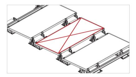
ATTACH LUGS: Use approved lug(s) to install on adjacent bays where the module is being removed.
