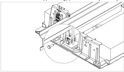
**INSERT COPPER WIRE:** Insert bare copper wire into each lug, providing a bonding jumper across the missing module location. Remove module & reverse the operation after maintenance is complete
