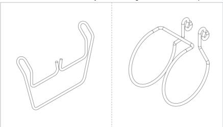
**OPTIONAL MICROINVERTER MOUNTING:** Microinverter / Power optimizer bracket, see page 9 for additional instructions.
