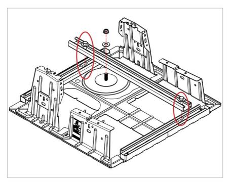
**STEP 4 – SECURE UNISTRUT TO ROOF ATTACHMENT:** Place 3/8" washer and 3/8-16 serrated flange nut on anchor stud, serrations facing down and tighten to 30 ft-lb.
