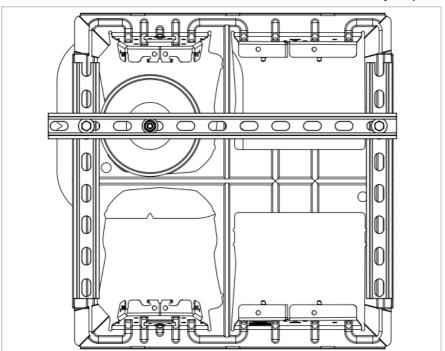
**STEP 3 – PLACE UNISTRUT:** Position strut sections on bay as pictured above. Align the cross-strut with the anchor's stud. Connect side strut sections to cross strut using a strutnut, bolt, and washer as pictured. **NOTE:** Metal base of attachment where stud is located cannot exceed a height of 1/4".
