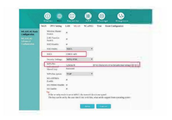
After the modification is completed.click "SAVE to save t and complete the modification af the wifi name and password
