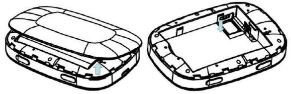
3. Insert the SIM card into the slot until it is fully inserted.
