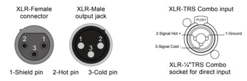
The unbalanced connection, pin-2 is hot, pin-3 is shield paralleled with pin-1.
