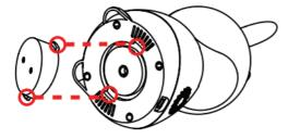
• Rotate the camera clockwise to slip into the bracket and secure the camera in position.
