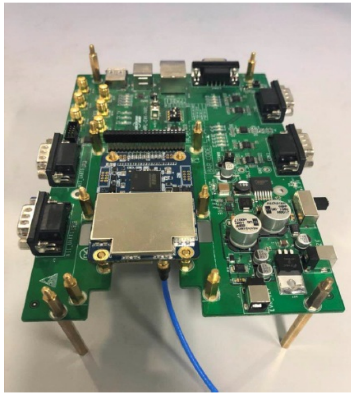
Figure 4-2 UB4B0M Connecting to Antenna RF Wires
