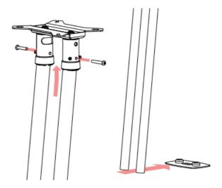
• Using the markings from Step 3, secure the floor plate into position. (Fixings not supplied).
