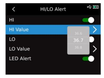
When the temperature of the measured object exceeds the high-temperature alarm temperature value, the red positive triangle will pop up. When the temperature of the measured object is lower than the low-temperature alarm temperature value, the green inverted triangle will pop up.
