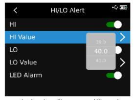
When the measured temperature exceeds the HI value, a red triangle will pop up. When the measured temperature is lower than the LO value, a green inverted triangle will pop up.
