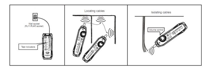
If the target cable are intermixed with massive cables, turn the sensitivity knob to adjust the sensitivity. Louder sound means stronger signal and closer to the target cable.
