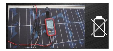
There is no requirement for batteries as the measurement can be effortlessly performed for extended periods.
