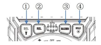
Selection key: Pressing this key can switch between the gear modes currently indicated by the knob switch, as follows:
