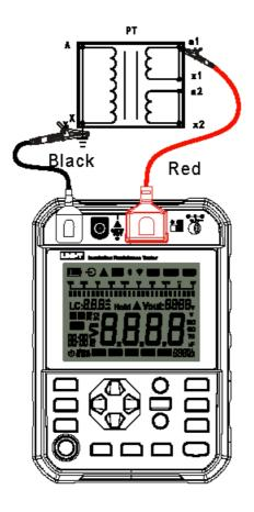
Fig. 10.2.2 Connection of testing
