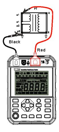
Fig. 10.2.3 Connection of testing
