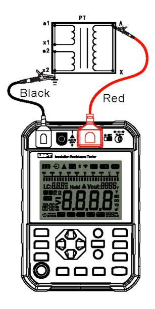
Fig. 10.2.1 Connection of testing
