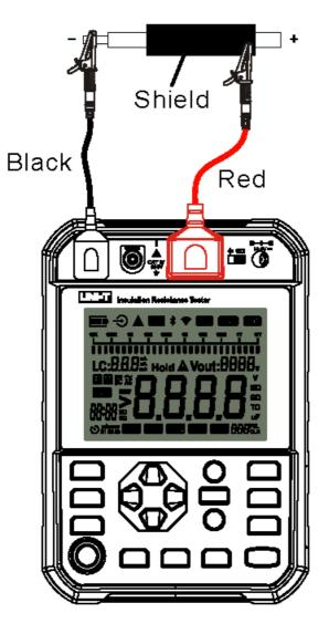
Fig. 10.1.1 Two-wire connection
