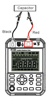
Fig. 9.3.3.1 Wire connection of capacitance measurement
