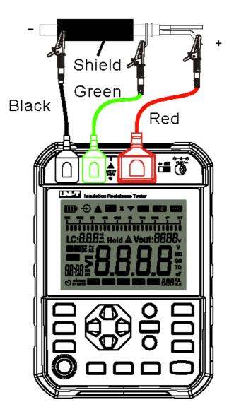
Fig. 10.1.3 Three-wire connection
