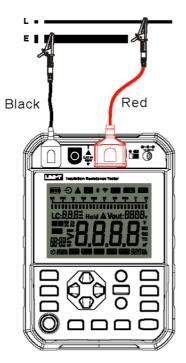
Fig. 9.3.2.1 Wire connection of voltage measurement
