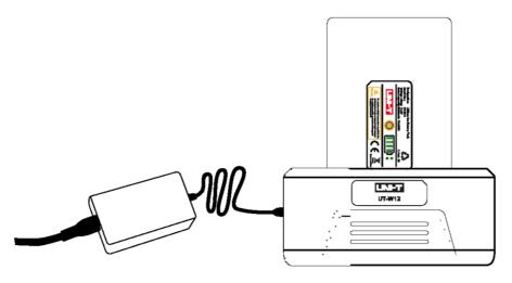
Fig. 9.2.2 Charged with charging stand (optional: UT-W12)
