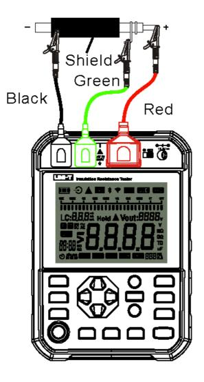
Fig. 10.1.2 Three-wire connection
