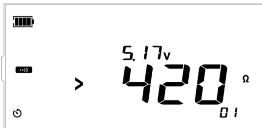
Figure 13.19 Low resistance exceeds the range
