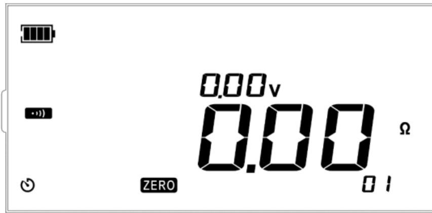
Figure 13.17 Resistance of shorted test leads is zeroed
