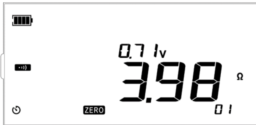
Figure 13.18 4Ω resistance measurement (Internal resistance zeroed)
