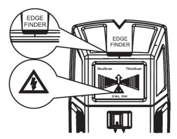
Both the StudScan and ThickScan modes can detect live AC wires, the maximum distance of detection is 50mm. When the device detects a live wire, the live hazard symbol appears on the LCD and the red LED light is on.
