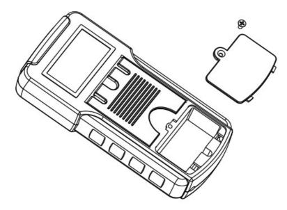
2. Load the 9V battery into the battery compartment correctly, close the cover and tighten the screw as the figure:
