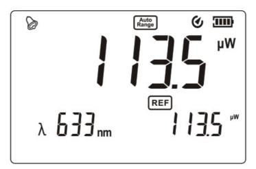
The short press REL button can enter relative value mode. It will subtract the relative value from the actual measuring value, the difference will be displayed in the main display area as shown in the figure:
