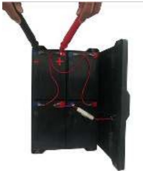
Figure 3-2-b Schematic Diagram of Crown Probe Test Pen Measurement
