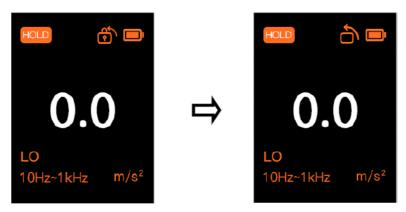
Lock the screen direction Unlock the rotatable screen
