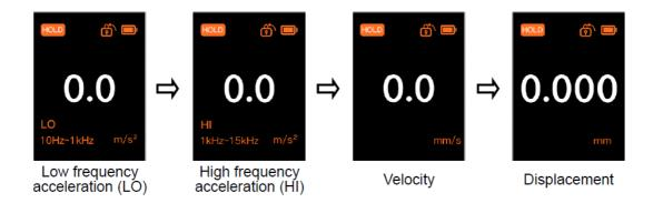
Low frequency acceleration (LO) 10Hz~1kHz m/s²→ High frequency acceleration (HI) 1kHz~15kHz m/s²→
