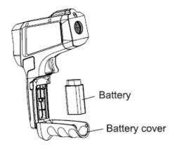
Install or replace a 9V battery (1604A) according to the following steps:
