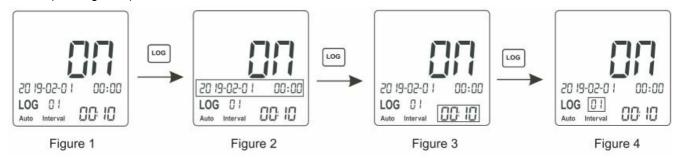
d) After setting the parameters, press the SET button or pull the trigger to return to the HOLD interface. The Auto Interval icon will flash.
