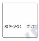
In the HOLD interface, press the SET button for 3s to enter the lock measurement setting interface, and short press the SET button twice to enter the system time setting interface. Short press the LOG button to select "Year - Month -Day -Hour -Minute" in turn and set the corresponding parameters.
