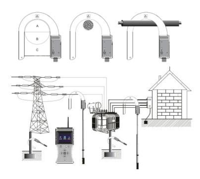
• Hook the neutral and live wires together to measure single-phase leakage current of electrical appliance.
