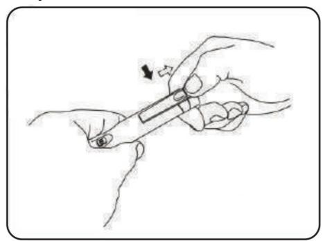
2. Please take out the upper cover of the test pencil according to the direction shown in the picture, and replace the battery. (see the following picture)
