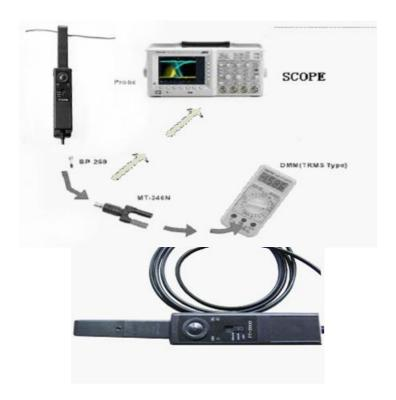
The current probe enables a general purpose oscilloscope to display AC and DC current signals up to 30 amps Peak (21A RMS). The current probe can also make AC and DC measurements with a multimeter by using the recommended accessory MT-246N (BNC-to-banana) plug adapter.
