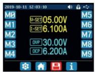
Press SHIFT + 0 to enter the system settings menu. Now press the right arrow key twice to call up the settings menu for data storage. Use the direction keys to select the desired data group. I-SET: Setting the memory output current V-SET: Setting the memory output voltage SHIFT + I-SET: Setting the memory overcurrent protection limit SHIFT + V-SET: Setting the memory overvoltage protection limit
