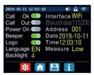
Press SHIFT + 0 to enter the system settings menu. The desired setting can be selected using the direction keys. The current selection is highlighted in red. The setting can be changed by pressing the encoder.
