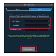
Now enter the WiFi name and password of the WiFi network to which you want to connect the laboratory power supply unit.
