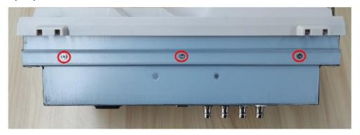
3. Use a PH1 Phillips-tip screwdriver to remove the two screws on the left and right sides.
