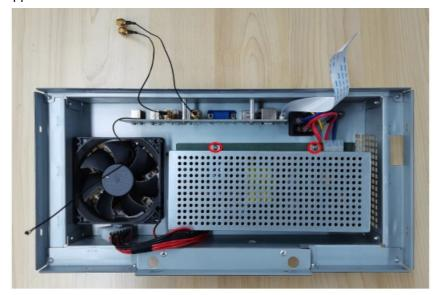
2. Use a PH1 Phillips-tip screwdriver to remove two more screws from the rear assembly and remove the power supply cover
