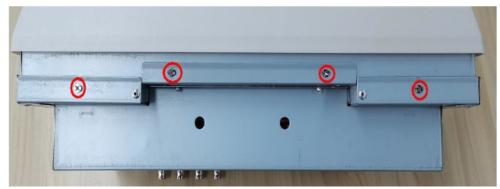
2. Use a PH1 Phillips-tip screwdriver to remove the lower three screws
