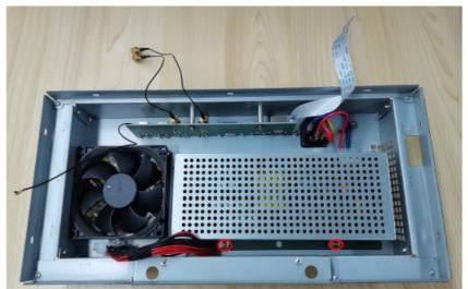
3. Remove the power cable and the fan power cable, then use a PH1 Phillips screwdriver to remove the four screws on the power module, and finally remove the power module
