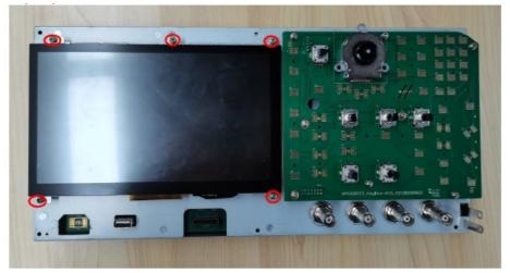
2. Turn over the display screen and fixing bracket, and manually remove the FPC cable from the display adapter board.
