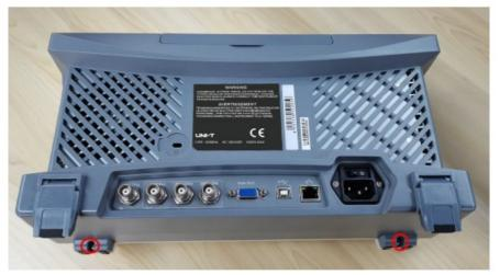
3. To reinstall, reverse the above steps. Use a PH1 Phillips-tip screwdriver to secure the screws
