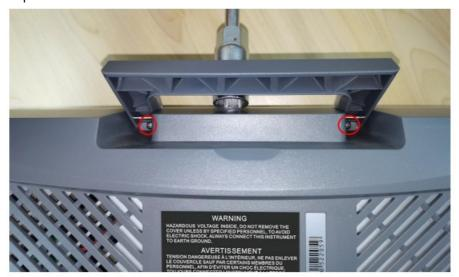
2. Remove the other two screws from the bottom of the case near the feet, and remove the rear cover.
