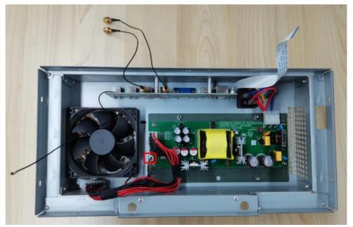
2. Use a PH1 Phillips-tipped screwdriver to remove the four screws from the back of the rear chassis frame and remove the fan
