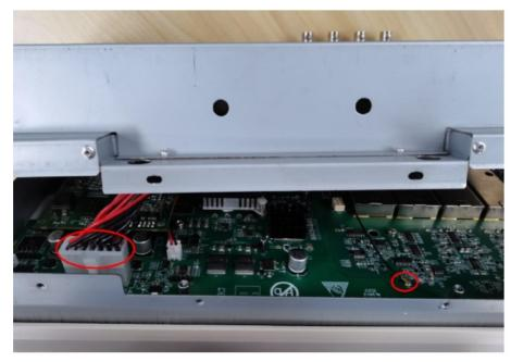
5. Flatten the front and rear components, and manually remove the connections of the coaxial cable on the signal source sub-board and the FPC cable on the main board.
