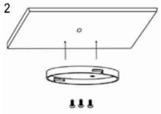
Install tack of the future to crating or wall and connect wires.
