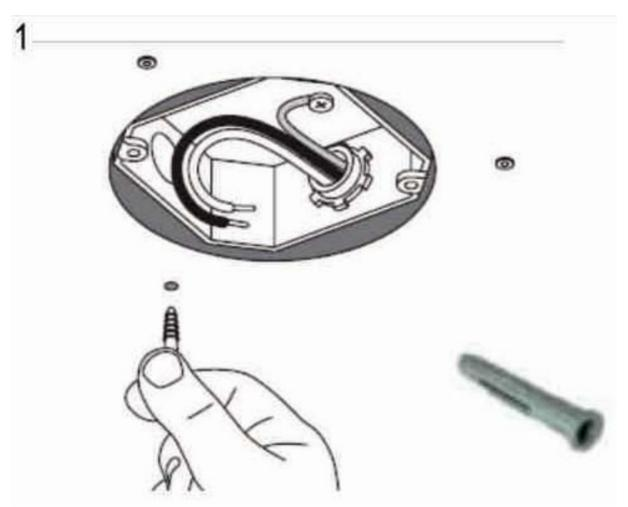
Prepare 3 h0les and install screw anchors.
