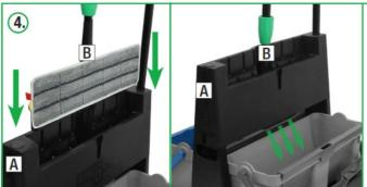
(EN) Insert mop (B) into wringer (A), wring mop 2x making sure to completely pull mop (B) out of wringer (A) each time. NOTE - Push/pull mop (B) vertically to insert and remove. DO NOT move it from side to side. This could damage the mop (B).
