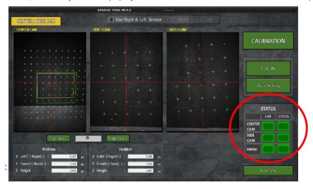
4. Use the "CENTER CAM" as your point of reference. Make sure the arrow on the calibration board is facing the impact screen. Align the crosshair on the calibration board with the red crosshair on the "CENTER CAM." (Double click the "CENTER CAM" box to enlarge image.)
