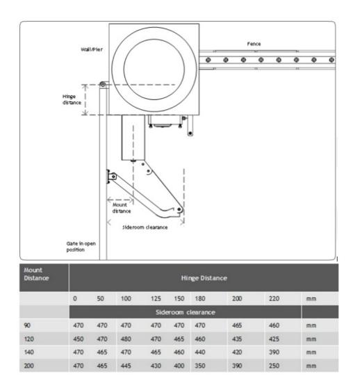
The mount distance for the drive unit and the hinge distance for the gate can be selected to opti-mise the side room clearance. See Fig. 02.
