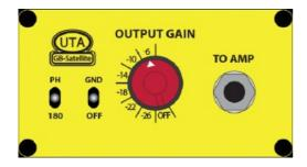
Connect the "TO AMP" output to an additional amp so you can layer the sound of multiple amps or easily A/B between them. Set the grounding switch to the "OFF" position to isolate the grounding of that amp. Use the phase switch to reverse the phase of that map.
