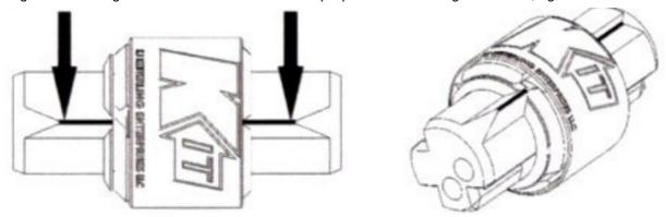
4. Insert stripped wires into opposing ends of connector. When properly inserted the wires insulation will be inserted into the housing approximatety 1/4".
