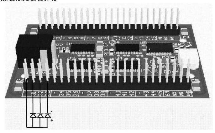
**Note** that if using Ultimarc Ultralux RGB pushbuttons, no additional connectors nor wiring is required. These have built-in wiring and connectors available in 2 lengths. The pins labeled A1-A6, PR, NX and GND are for future customized OEM versions of the board and are not used in the standard version.
