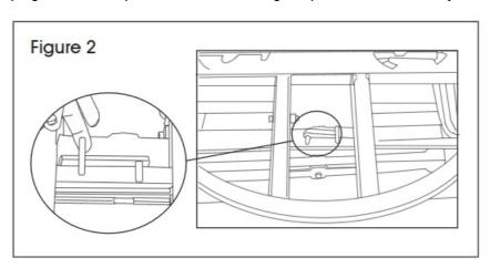
5. While keeping the platform raised, place the pin from step 2 into the hole in the roller track closest to the hinge. (See Figure 3)
