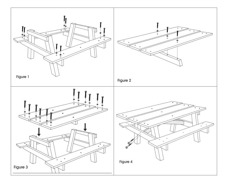
NOTE: It is important to keep the lag screws loose throughout the assembly. Tighten during step 8.
