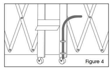
**CAUTION!** Notice that the center drop pin at this stage hits the other half of the gate or rests on the floor. Do not cut off the drop pin.
