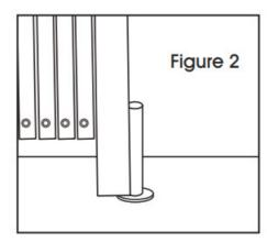
2. Have a helper extend the gate and stand it upright where it will be mounted. Drill 3/4" diameter x 3" deep hole, 1/" from the wall into the floor for gate pin to set into. Place a bearing washer over the floor hole and set the bottom gate pin into the floor mount hole. (See Figure 2)
