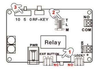
1. Lock Mode Select NO: Fail-Secure Lock NC: Fail-Safe Lock
