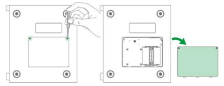
2. Unscrew the M.2 fixing screws.
