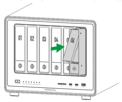
Por installing 3.5-inch hard drives, please remember to move the fastening pin back to the rear end.
