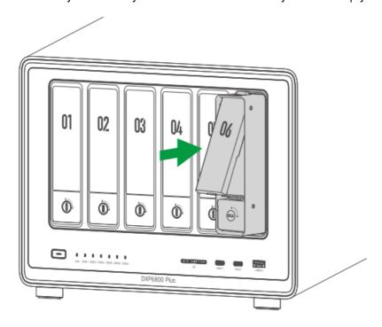
**Installing 2.5-inch Hard Drives (Screwdriver Required)**
