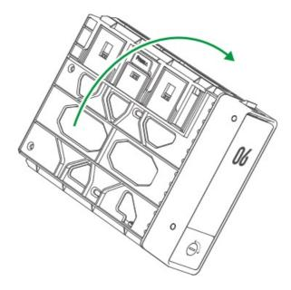
2. Pull the clamp arm: Press the buckle marked with the "Press" icon to pull the arm.
