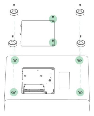
3. Turn to the back of the device, then remove the screws that secure the back ventilation cover.
