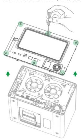
4. Remove the internal fixing screws that secure the outer shell to the internal frame, then lift the shell off the device.
