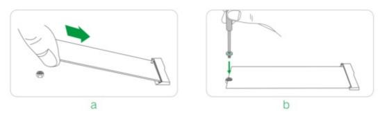
4. Peel off the protective film of the silicone pad and stick it on the front-facing surface of the SSD, then peel off the film on the other side.
