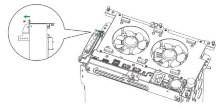
6. Insert the card into the slot and ensure the card is connected securely, then tighten the screws.
