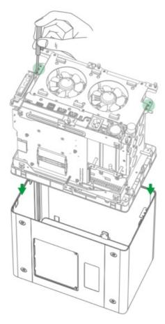
5. Remove the screw on the existing bracket. Then remove the bracket and keep it in case you need to replace the PCIe expansion card.
