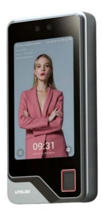
Uface 5 Pro series is a versatile intelligent terminal that supports rich extensibility, an optional QR Code and Fingerprint module, offering the IP65 waterproof protection for an outdoor solution.
