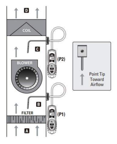
Static pressure testing ensures if the equipment is operating within factory specifications.
