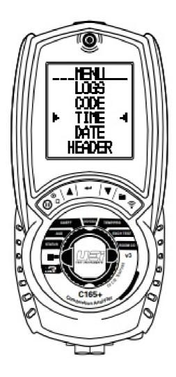
Press "Power" Button for 2 seconds. The analyzer will perform a 60 second purge. This should be done in fresh air.
