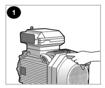
Ensure a clear passage using a manual grease gun. Remove any hardened grease by purging the lube point with a grease gun.
