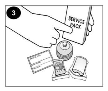
Insert battery pack and grease cartridge inside the M-UE. Prime the cartridge by lightly squeezing it until a quarter-inch of grease is visible out of the tip.
