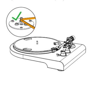
• Slowly rotate the platter ten times in the direction of the arrow for resetting the auto mechanism to avoid any twists in the belt and make sure the belt rides smoothly along the drive rim on the underside of the platter
