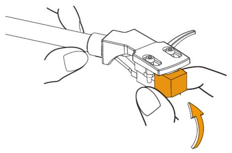
3. Make sure there is no gap between the headshield and the cartridge.
