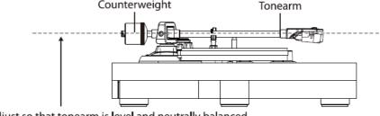
Adjust so that to nearm is level and neutrally balanced
