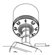
7. Rotate the counterweight counter clockwise (as seen from the front) to adjust the tracking force according to the cartridge manufacturer's recommendations.
