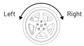
• Turn on the high lights by twisting it right to hold for a maximum of 3 seconds.
