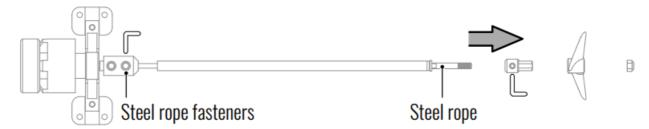
• **Installation:** Replace the new steel rope, the installation step is opposite to the removal step.
