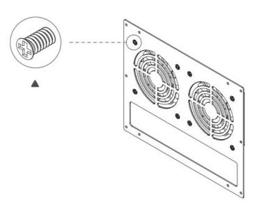
3. Install two frameworks to the back panels. Please note that all the screws for the enclosure are M3 \* 4 countersunk screws.
