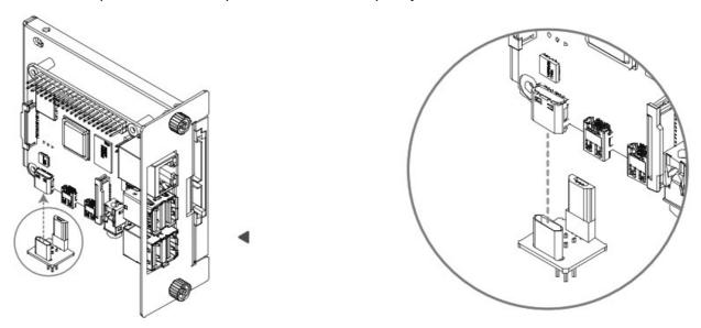
12. Polarity diagram of fan adapter.
