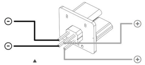
13. Connect the fan wire to the fan adapter board. Please pay attention to the red-and-black wires. Red represents the positive pole and black represents the negative pole.
