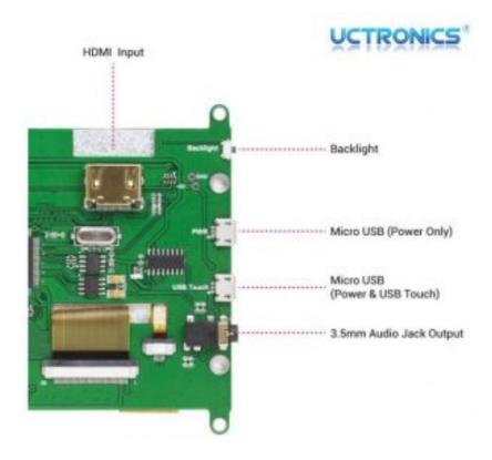
The connectors on the back of the display
