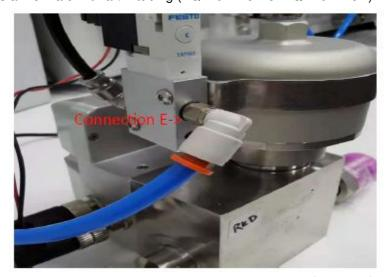
Warning! The solenoid requires the supplied gas pressure to be from 70PSI to 90PSI (5 to 6 BAR).
