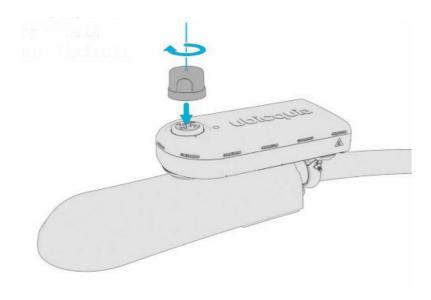
**CAUTION**: The UbiHub does not need a photocell to function, but should always have something installed in the NEMA. Never leave the top NEMA socket open.
