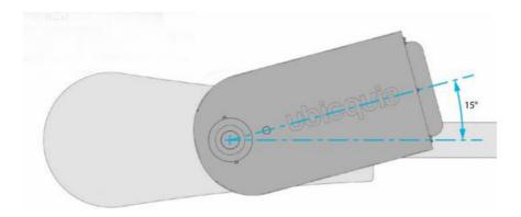
6.4 Once plugged, rotate the UbiHub towards the pole to lock the NEMA connecter in place. Stop once the clamp is aligned with the pole.
