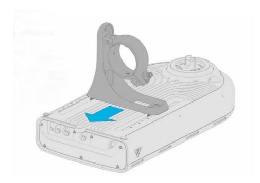
**NOTE**: If clamp placement was premeasured, or if installing multiple units on the same luminaire type, set the clamp position using the reference dimensions on both the housing and clamp, then tighten all adjustment bolts to 40 in-lbs torque.
