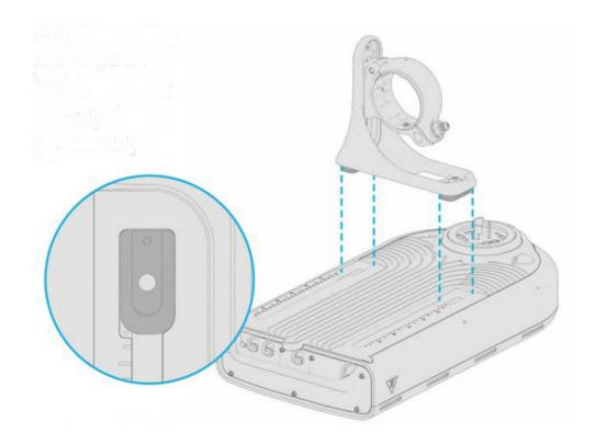
3.6 Slide the clamp along the housing rails and hand-tighten into position for now.
