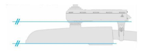
6.7 A. Once unit is leveled, tighten the vertical adjustment screws to 40 in-lbs torque using the 3/16" Hex bit driver.
