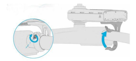
6.6 Adjust the clamp vertically as necessary to ensure the device is parallel with the bottom of the luminaire to ensure there is no undue stress or strain on the NEMA socket.
