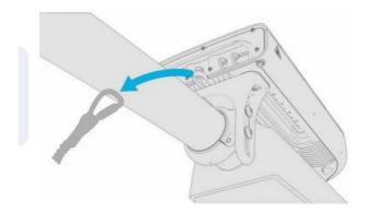
**NOTE**: Remove all protective packaging material from the camera prior to installation.
