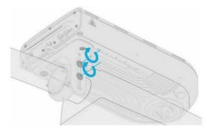
B. Then tighten the horizontal adjustment screws to 40 in-lbs torque using the 3/16" Hex bit driver.
