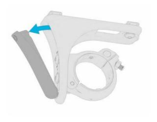
3.5 Align the shuttles on the top of the clamp with the rail openings on the bottom of the UbiHub housing while still in the box. There is a single orientation for assembly.
