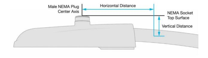
**NOTE**: Record position horizontal and vertical dimensions on UbiHub and clamp for later use in multiple installations of the same luminaire type.
