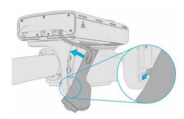
6.10 Tighten the camera top screw to 15 in-lbs torque using the 3/16" Hex bit driver.
