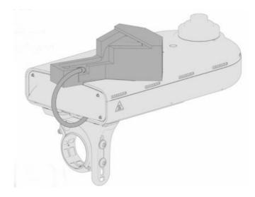
**NOTE**: The camera is shipped wrapped in protective packaging and connected to the unit. Do not remove the protective packaging until instructed to.
