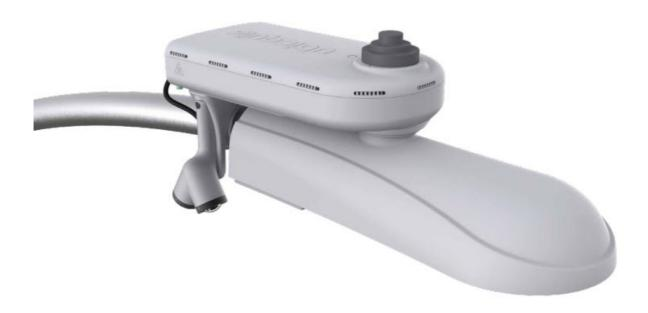
**CAUTION**: Double check the mounting bracket is snug and secure and ensure the blue films have been removed from the camera lenses and top light sensor.
